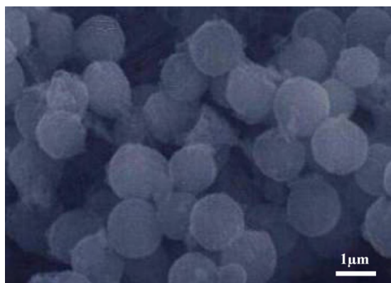
Fig. 12. SEM micrograph of the PMMA-silica microsphere with unmodified PMMA.
